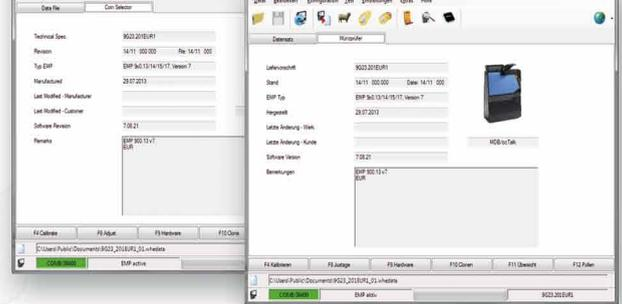
Wheasy 5 is a user friendly Windows™ software for testing and programming our electronic coin selectors from version v6 onwards. The existing settings of the coin selector may be read, changed and tested by means of a standard PC or notebook.
